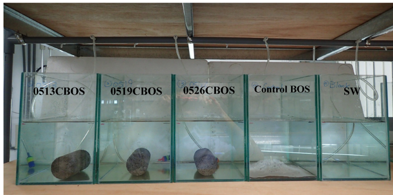
Fig.6. Experimental apparatus of BOF slag immersed in sea water.
