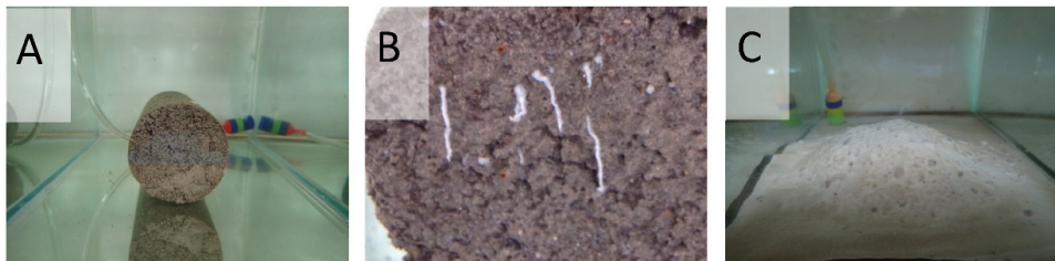
Fig.8. Surface conditions of carbonated BOF slag
