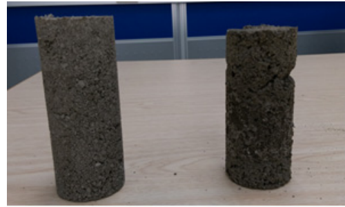
Fig.4. Appearance of Carbonated BOF Slag.
